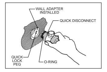
Take the Wall Fitting and Twist Lock the Wall Fitting into the Wall Adapter 1/4 turn and pull out, to a snug fit. Once the Wall Adapter is secure, you can now twist lock and unlock to remove Wall Fitting with ease from the Wall Adapter.
